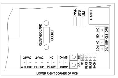
Once the device has been powered up the RED indicator on top of the newly installed receiver card should light up and remain lit. This indicates there are currently no transmitters installed. *If the RED indicator does NOT remain lit you should preform a 'bulk erase' (see next page).*
