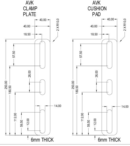
BOLTS FOR AVK HAVE RUBBER SHRINK WRAP ON THREADS SO THAT METAL TO METAL CONTACT DOES NOT OCCUR BETWEEN MOUNTING PLATE AND MOUNTING BRACKET.
