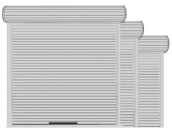
Door height: 4.5m, 3.0m, 2.3m Door width: 5.4m, 4.0m, 2.2m Single dwelling, max door weight: up to 80kg
