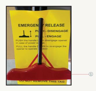
• To disengage BRD9 unit push the **red handle** upwards, and you can then operate the door in manual mode. To re-engage the unit pull the red handle downwards.
